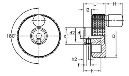
$$\begin{array}{lll} D & = 40 & L = 20 \\ d1 & = 17 & I2 = 7 \\ d2 & = 14 \\ d & H9 = 6 \\ f & = M4 \end{array}$$
